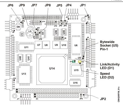
Figure 2-5. Jumper and LED Locations (Top View)
